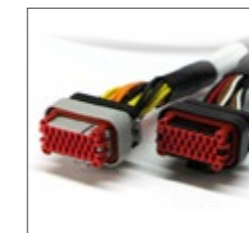
M812 Connector Harness (Part No. 016-185) Set of 2 coded AMP SEAL connectors pre-wired with 1.2 metre cable.
